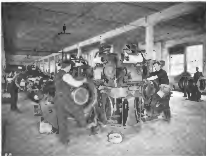
How the Goodyear Tire Machine Stretches the Fabric
